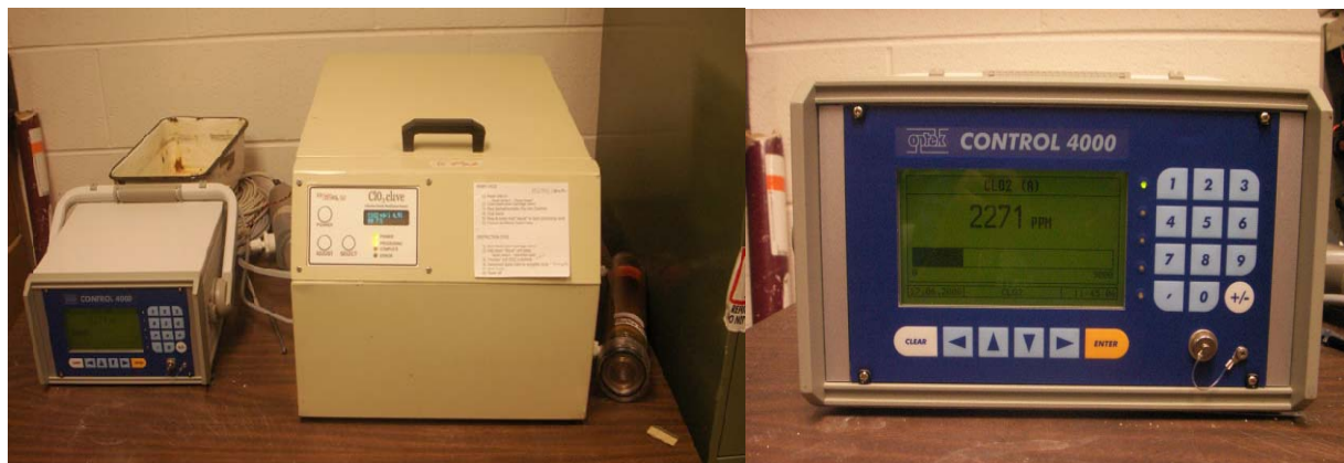
Figure 22. ClO 2 Clave for chlorine dioxide treatments and measurement of chlorine dioxide gas in ppm.
